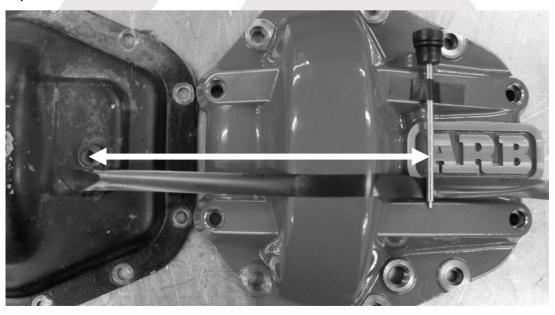
Using a file, clearly mark the dipstick at the desired fill level so you can effectively oil fill to that mark later.
