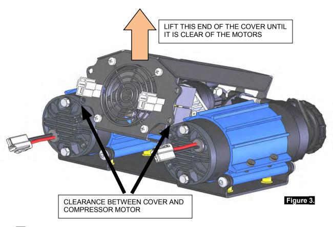
Slide the cover towards the intake filter end to unhook the cover from the compressor head.
