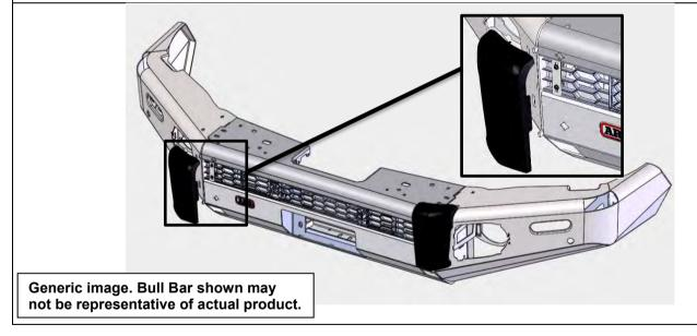
62. Ensure each buffer sits flat against the face of bar. Secure wing side using retaining clips. Secure inner side using the angled cup washers, flat washers and screws.
