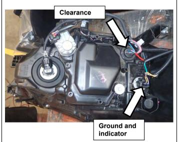
20. Following fitting instructions 3789197 supplied in kit 6821287; attach the LED combination lamp looms (also supplied in same kit). Vehicle coloured wires can be found in the positions indicated.
