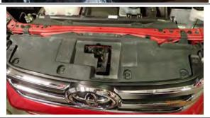
94. Re-install upper radiator cover panel and fasten using 8 x OE scrivets.
