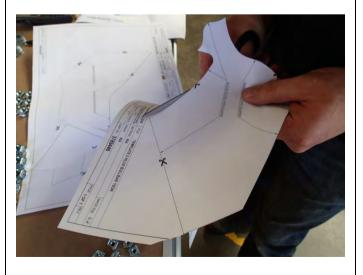
22. Carefully cut out both bumper cut templates supplied.
