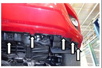
Remove all fasteners and scrivets retaining bumper along lower lip – (Left Hand side shown).
