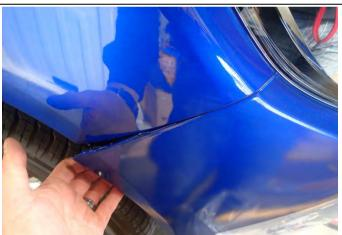
10. Remove registration plate and set aside, then carefully remove bumper from vehicle by pulling on each side of the bumper near the wheel arches and working your way towards the centre.
