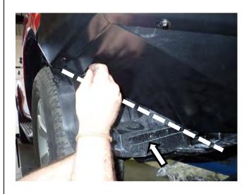
83. Mark lines onto the OEM inner guards (LH & RH) using lower edge of wing under panels as guide ensuring enough guard remains so that it may be neatly tucked/secured behind wing under panel lip.
