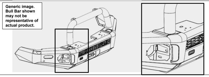
66. Fasten top tube to the bar using 4 x M10 SEMS Bolts. Adjust position of top tube left/right until it sits central on the bar and the rear buffers are positioned correctly. Tighten M10 SEMS Bolts to specification. Tighten Rear buffer screws.
