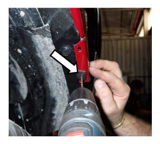
88. Install scrivet clip onto inner guard and bumper outer end as shown.
