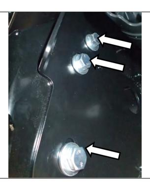
70. Loosely fasten bar to mounts using 6 x M12 x 1.75x35mm bolts, 6 x M12 spring washers, 6 x M12 flat washers (4mm thick) and 6 X M12 flange nuts.
