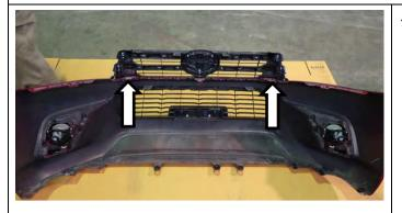
18. Remove grille from bumper by carefully releasing locking tabs whilst removing.
