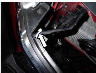
38. Cable tie the air deflector panels to the grille. (RH shown).
