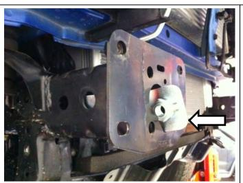
39. Insert 2 x M12x1.75 nut plate into RHS chassis rail as shown.
