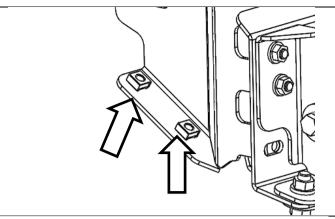
81. Fit 4x M8 cage nuts to RH and LH bull bar mounts as indicated. (RH Mount Shown)
