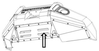
82. Fasten stone tray using 4x M8 bolts, flat washers and spring washers and 2x M6 OEM fasteners
