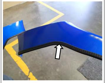
34. Apply bumper trim pinch weld to both RH and LH sides along the full length of the cut edge. Carefully trim off any excess length.
