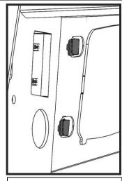
Slide retaining clips through tabs to lock buffer in place
