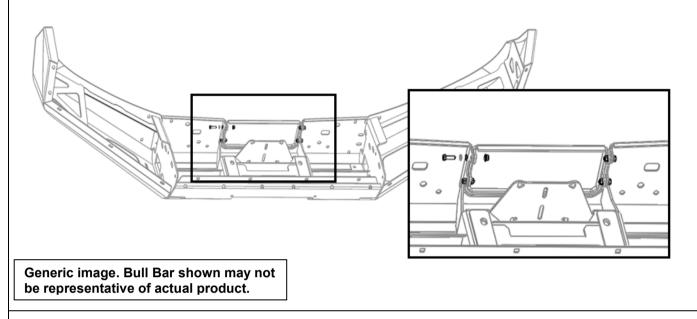
52. Fit the number plate bracket to the top face of the lower-centre pan on the bar using 3 x M6 x 20 hex bolts, spring washers, flat washers and flange nuts.
