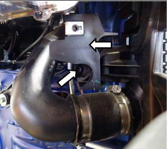
Remove M8 fastener from upper crush panel support brackets. Remove support brackets from vehicle and discard. (Right hand side shown).
