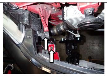
2. Remove lower grille retaining screws – (Right hand side shown).
