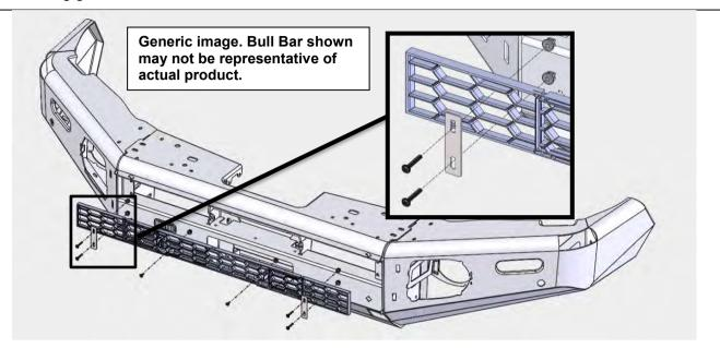
61. Place each of the front buffer sections onto the bar as shown. Ensure that the 2 lugs and 2 screw bosses pass through the holes in the bar.
