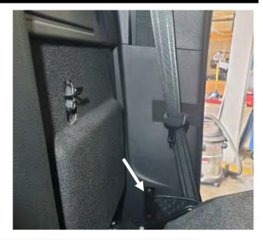
Reinstall the plastic trim. Bracket should be positioned as shown. Reinstall door jamb seal and scuff plate.
