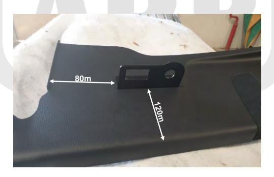
Lay the trim down and position the bracket as shown. Mark the mount holes with a permanent marker.
