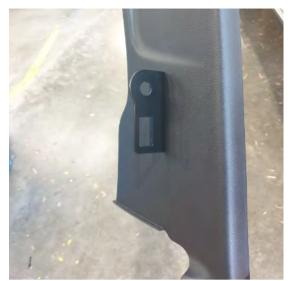
Drill out the mount holes to 7mm. Mount the bracket as shown using 2x M6x20 bolts, M6 flat washers & M6 flange nuts.
