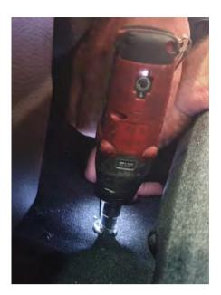
If using the supplied nutsert tool, hold the lower machined nut with a 12mm spanner. Tighten the M6 bolt with a 10mm socket & ratchet or using an impact driver as shown.
