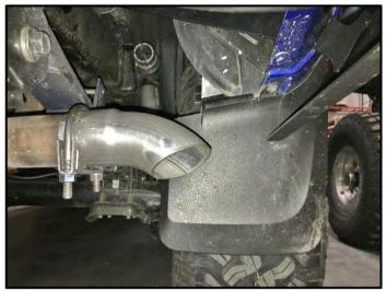
57. Cut the exhaust back at it's end, and install the supplied exhaust tip leaving a good distance between the tip and the wing panel. A high temperature paint can be used to avoid corrosion if desired.
