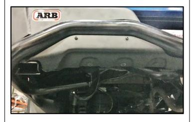
54. Install the bottom diffuser panels using the supplied (6) M6 black button head bolt and flat washer sets. The bottom outside corner attachment uses a flat washer and nyloc nut with the button head bolt.
