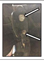
18. Remove the angle brackets on the bottom of each frame rail by removing the (2) hex screws shown on each side. Discard these brackets.
