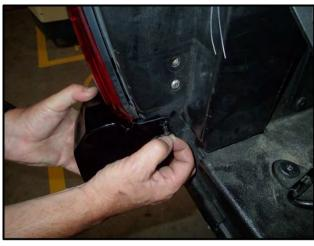
37. Secure the inside edge of the corner caps to the vehicle using the plastic rivet from the OE part, as shown in the diagram.
