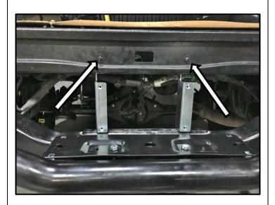
40. Secure the (2) beaver panel support brackets through these holes, using the supplied M6 hex bolt, spring washer, and flat washer sets.
