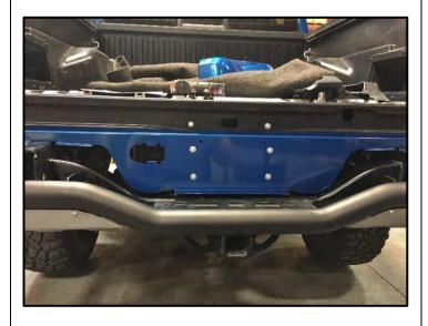
41. Temporally fit the beaver panel to the support brackets with (4) M6 button head bolt, and flat washer sets.
