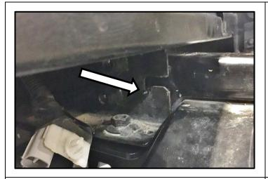
Remove the receiver hitch and bumper in one piece from the truck by unbolting the (7) hex bolts from each side and removing.
