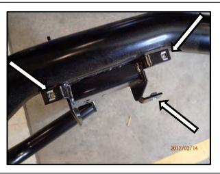
17. Install (6) long leg M6 cage nuts into the bar assembly at the locations shown in the picture.
