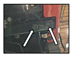
10. Starting with the left side, remove the (2) hex bolts on the underside flange of the receiver as shown in the picture.
