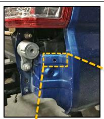
32. Mark and drill an Ø 8mm hole 15 mm from upper edge and 15mm from inside edge as shown. Repeat on opposite side.
