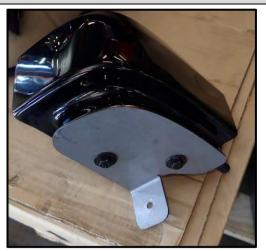
31. Assemble the Rear Quarter Cap and mount bracket with (2) M6 hex bolts, flat washers and nyloc nuts.
