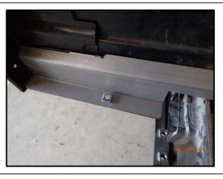
42. Fit (2) short leg M6 cage nuts to the beaver panel outside flanges. Note that the nut should be on the top side of the flange.
