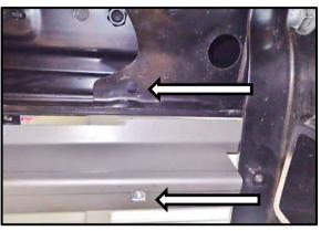
43. Using (2) M6 hex bolt, flat washer, and nyloc hex nut sets, fit the outer beaver panel mount brackets to the chassis and beaver panel.
