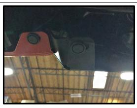
8. Remove the (4) plastic clips on the underside of the bumper fascia.
