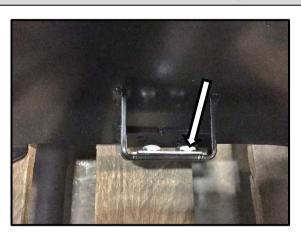
44. Insert the plate nuts into the wing panels inside tabs as shown in the picture. (1) plate nut per wing.
