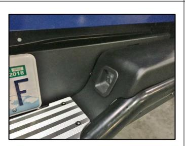
51. Adjust the wings so that the gap between the wing and the beaver panel are parallel. Ensure that the gaps between the wings and fender panels are even. Once you have achieved the gaps and margins required tighten all nuts and bolts to required torque settings.
