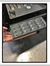
9. Pull off the tread plate portion of the rear bumper by starting at the ends and prying up. This part will not be re-used, but to avoid cracking this part, be sure to not use excessive force during this operation.
