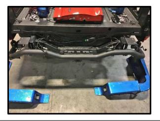
26. Before installing wing panels reconnect the wiring harness (from step 1-2) and ensure that all connection terminals are in the correct areas to reconnect to the corresponding sensors.
