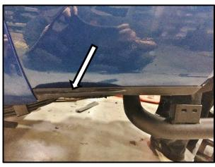
19. Remove the (2) plastic covers on the bottom of each fender if equipped.
