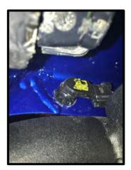
27. Reattach the re-located sensors to their correspoding wire connectors.
