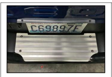
50. With the aluminum tread plate secure the inside flanges of the wings to the top of the frame using (4) Stainless (silver) button head bolts.
