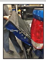
3. Remove the tailgate from the truck by unhooking the support cables on each side. Bring the tailgate to roughly a 45° angle and pull rearward on the passenger side. Once the passenger side hinge is released pull tailgate to the right to release it from the left side hinge. Be sure to carefully push the wiring harness through the cutout in the truck body before walking away with tailgate. Place in a safe place to avoid damage.
