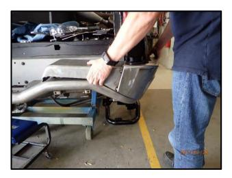
45. With the help of another person. Starting with the driver side, position the wing onto the tow bar.
