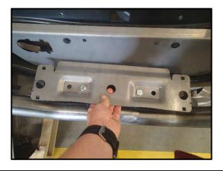
30. Place the frame mount plate from the previous step over the (2) spacers. Hand tighten (2) M10 x 40mm Hex Bolts, and Flange Nuts sets, securing the frame mount plate to the plate on the ARB bar frame.
