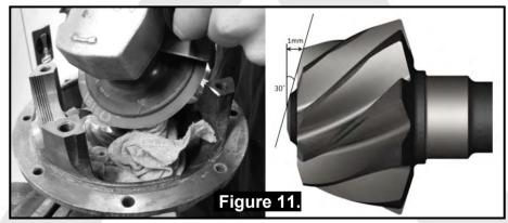
☐ Check clearance again using a feeler gauge and remove more material if required. The modified pinion should look like figure 12...
