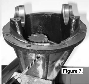
☐ Tap the hole from the outside using ¼"NPT thread tap.
