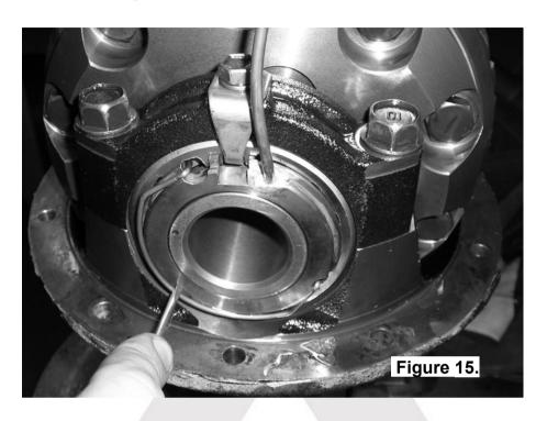
☐ Check that the seal housing is now secured from rotating and that it is still sitting flat against the adjuster nut.
