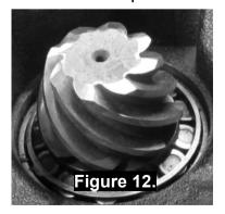
NOTE: Modifying the pinion gear in this way does not weaken the pinion at all.
