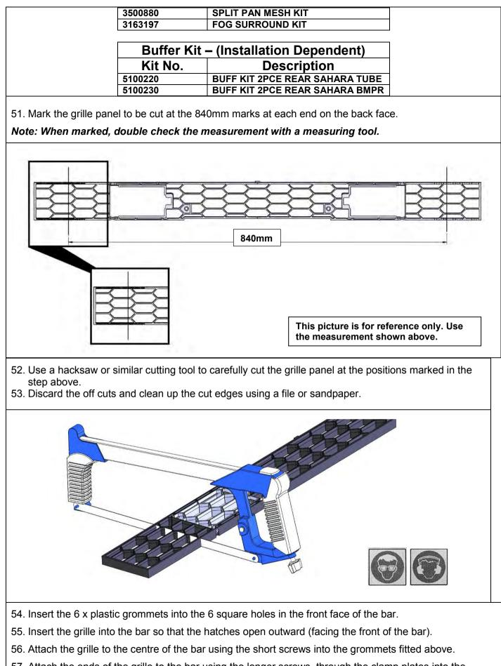
57. Attach the ends of the grille to the bar using the longer screws, through the clamp plates into the remaining grommets.
