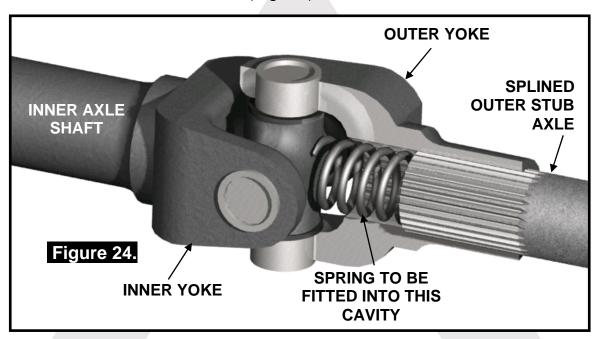
NOTE: When assembled, ensure that the spring maintains sufficient pressure on the axle to hold it firmly against the cross shaft of the differential while the vehicle is sitting on level ground.
