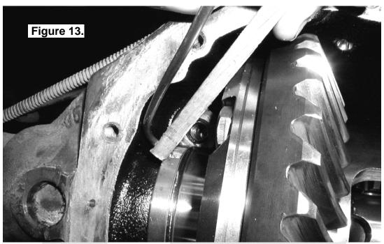
NOTE: The seal housing tube should lay as low in the seal housing groove as possible.
