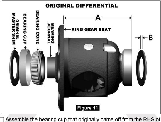
Assemble the bearing cup that originally came off from the RHS of the differential carrier onto the bearing cone on the RHS.
