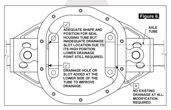
If no drainage exists at all then slots or holes should be created in the bearing seat face of both axle tubes; one on the upper side of the tube, and one on the lower side.
