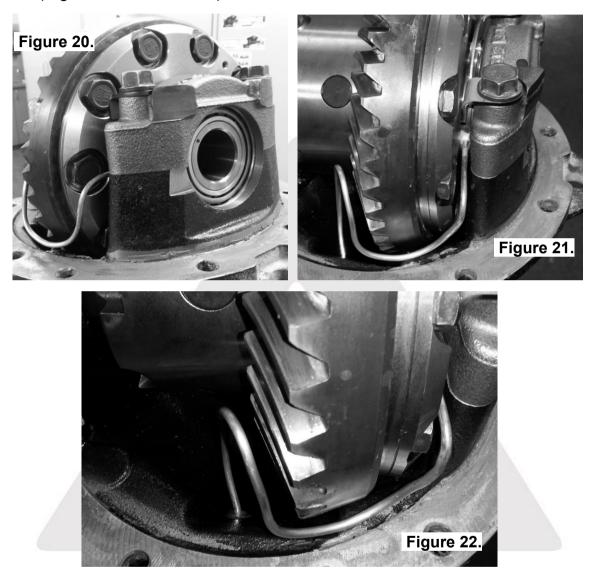
**NOTE :** It is a good idea to keep the tube away from the bearing caps or any other part of the differential casting as any contact due to vibration or shock may wear the tube and eventually cause a leak.
