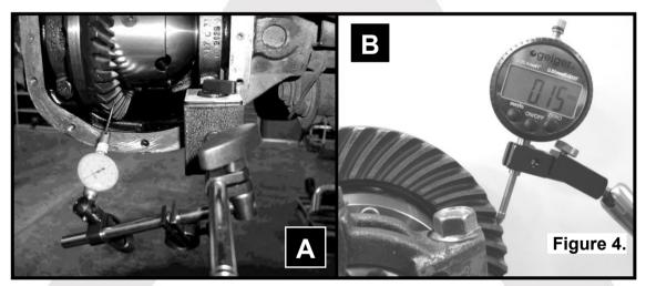
Set a depth indicator on one of the ring gear teeth as in figure 4.
