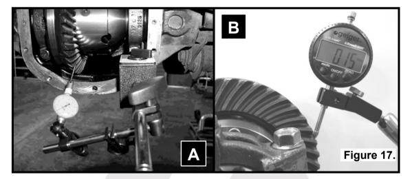
Refer to your vehicle service manual for the specified maximum and minimum amounts of backlash. If the backlash is not within the specifications then the differential will have to be removed and reshimmed.
