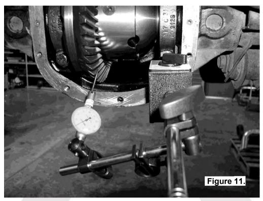
Refer to your vehicle service manual for the specified maximum and minimum amounts of backlash. If the backlash is not within the specifications then the differential will have to be removed and reshimmed.
