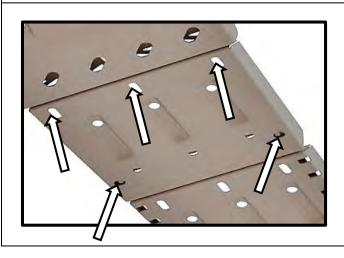
4. Hold the 2<sup>nd</sup> panel from the front up to the vehicle and fasten the (3) M8 x 25mm hex bolts, spring washer, and flat washer sets connecting this panel to the 1<sup>st</sup> panel. Fasten the (2) M8 x 35mm hex bolts, spring washer, and flat washer sets into the factory weld nut locations as shown. Do not tighten these fasteners at this step.
