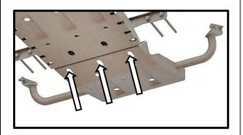
10. Hold the 4th panel from the front up to the vehicle and fasten the (3) M8 x 25mm hex bolts, spring washer, and flat washer sets connecting this panel to the 3rd panel. Do not tighten these fasteners at this step
