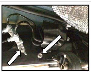
8. Remove the (2) hex bolts securing the fuel line bracket and cover shroud to the frame as shown in the picture (**note**: some variants of this truck do not have the fuel line shroud). Discard these fasteners, pull the fuel lines away from the frame to allow space for the 4<sup>th</sup> panel.
