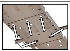
7. Hold the 3<sup>rd</sup> panel from the front up to the vehicle and fasten the (3) M8 x 25mm hex bolts, spring washer, and flat washer sets connecting this panel to the 2<sup>nd</sup> panel. Fasten the (2) M10 x 30mm hex bolts, spring washer, flat washer, and serrated nut sets connecting the 3<sup>rd</sup> panel to the crossmember brace installed in the previous step. Do not tighten these fasteners at this step.
