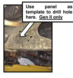
9. For Gen II Tacomas, the forward most hole is not predrilled into the frame of the vehicle. Using the 4th UVP panel as a template, match drill the frame to include these holes at Ø9.0mm.
