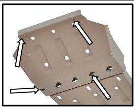
3. With the help of another person, hold the front panel to the vehicle and fasten (2) M8 x 25mm hex bolts, spring washer, and flat washer sets into the factory weld nut locations as shown in the front. Fasten the (2) M8 x 35mm hex bolts, spring washer, and flat washer sets into the factory weld nut locations towards the rear. Do not tighten these fasteners at this step.
