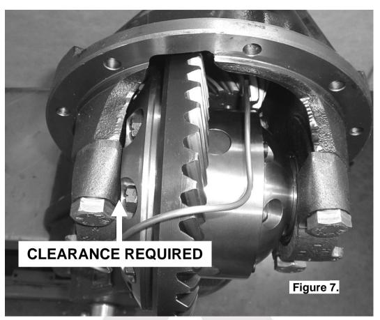
Insert the original adjuster nut onto the opposite side of the differential and tighten with the appropriate adjuster nut wrench.
