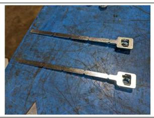
4. Position M10 cage nuts into nut plates as shown.
