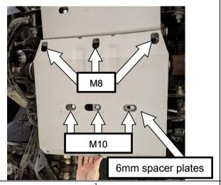
6. Loosely fasten ARB diff panel to vehicle and Front Panel as shown using fasteners supplied in kit. REFER "FIT DIFF PANEL" SECTION OF TABLE ON PAGE 3. Ensure to secure the 6mm spacer plates between the diff panel and chassis (as seen in the image below).
