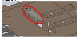
7. Loosely fasten ARB transmission/transfercase panel to vehicle and Diff Panel as shown using fasteners supplied in kit.
