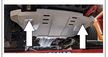
Remove factory front & diff stone guards from vehicle and set aside front 2 fasteners. 1.
