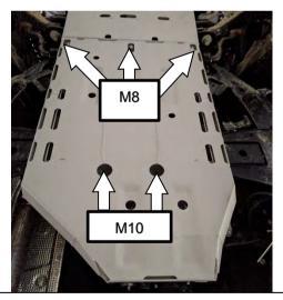
8. Tighten all fasteners beginning with sets fixing panels together and then move on to fastener sets fixing panels to chassis.
