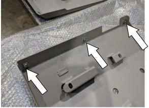
3. Position M8 cage nuts into front panel as shown.
