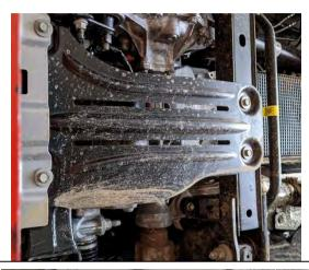
2. Remove factory transmission guard from vehicle.
