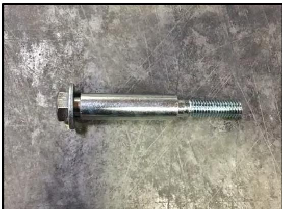
7. Insert the M12 x 110 hex bolt into the supplied 60mm crush tube with a flat washer. Feed this assembly through the rear most hole that was drilled to  $\text{Ø}18\text{mm}$ . Secure on the opposite side of the frame with a supplied flat washer and M12 nyloc hex nut.
