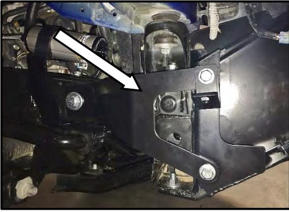
1. Remove either factory center stone shield or center stone shield and right wing panel of bull bar if already fit to vehicle. Remove stock air dam if equipped.
