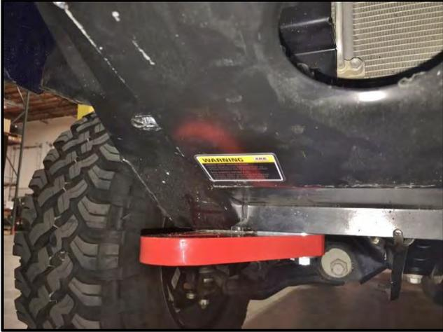
15. Install (1) supplied 'Warning Label' onto center stone shield as shown in the adjacent picture, or in plain sight onto stock air dam.
