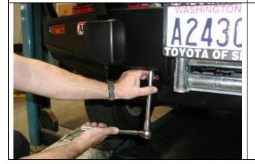
35. If driving lights are to be fitted, use extension bar with ratchet, 3/4" long reach socket to tighten from cutout in centre pan
