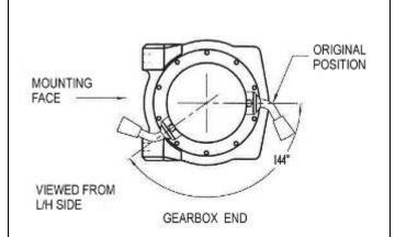
8. To place the clutch handle in the correct position, the winch gearbox must be rotated 144 degrees (4 hole spacings), in anti- clockwise direction when viewed from gearbox end. Place the winch on its end and remove all gearbox bolts. Gently raise the gearbox just enough to rotate it. When the correct position is located, refit all bolts and tighten.
