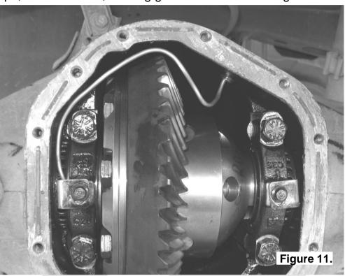
NOTE: Less than 8mm [5/16"] between the tube and ring gear should be considered too little clearance.
