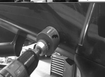
62. Using a Ø70mm hole saw, drill through the rear side panel using the mark from the previous step as the centre point of the hole.
