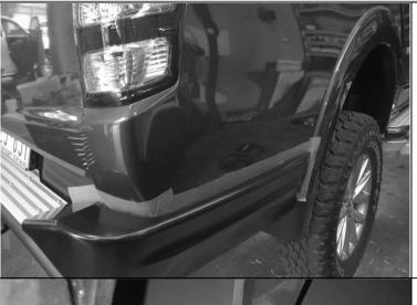
71. With the assistance of other people or a lifting device, position the Triton wing next to the rear side vehicle panels. Take care not to damage the vehicle when positioning the Triton wing.
