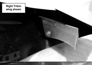
66. Fix a wing mount bracket to each Triton wing using 3 M8x1.25x25hex head bolts, 3 spring washers, 3 flat washers and a wing triple nut plate. Orientate each bracket as shown. Leave bolts finger tight at this stage
