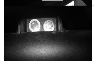
2 M8 bolts, 4 M8 washers and 2 M8 nyloc nuts
