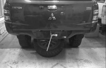
3. Remove the spare wheel from beneath the tub using the wheel nut wrench and jack handle pieces supplied with the vehicle. Insert as shown through the access slot above the number plate position and rotate counter-clockwise to release the wheel.
