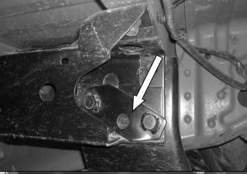
Remove bolt plate from inside of chassis rail from each side and discard as shown and remove bumper bar
