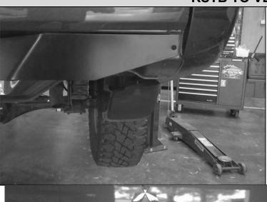
11. Attach beaver to rear of tub as shown using single M6x20 black button head fastener with black flat washer.M6 nyloc and flat black washer on tub inside face
