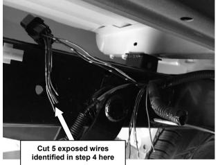
5. Cut a 90mm section from the centre of the 5 exposed wires. This will leave ~55mm of wire before they re-enter the corrugated tubing and the 8-pin connector.
