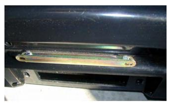
25. Secure the number plate bracket using M6 bolts, flat washers and flange nuts. Attach the longer side to the bullbar and the shorter side to the number plate.
