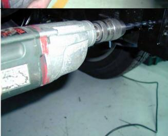
10. Then, as shown, using a Dia 10.0 drill, drill hole through inner wall of chassis.
