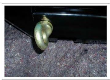
23. Screw in the eyebolt using the large washer. Eyebolt can be positioned to sit vertically by rotating the large nut to the correct position
