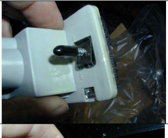
Remove lights from cartons and then remove screws and speed nuts from each light. These fasteners are not to be reused – new screws are supplied in the fitting kit
