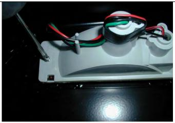
21. Fit lights using screws supplied in fitting kit, taking note of RH and LH light bodies, they are different and must be placed on the correct side of bull bar.
