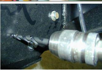
43. Using the M10 pilot holes in mount brackets, drill pinning hole through uprights on bull bar. Fit M10 screw, washer set and flange nut and do up tight.
