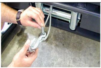
55. If winch fitted, fit off winch hook.
