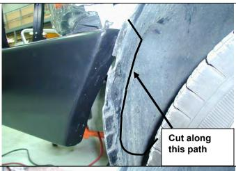
56. Trim fender liner with air hacksaw or similar tool along line as shown. Cut away the outboard flap, which normally fits in the end of the bumper wing. This is so the liner can be held back easily by the retaining bracket at step 56.
