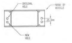
30. In some cases, the roller fair lead bracket must have a second set of holes drilled to line up with holes in winch bracket. If required, mark out as shown and using a 13.0 mm drill bit, drill two holes as shown in diagram.
