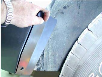
57. Fit liner retainer bracket with black M6 bolt and washer sets into M6 cage nuts in wing returns each side as shown.
