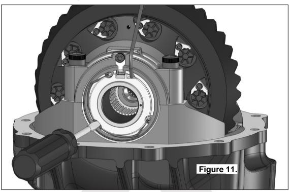
Check that the seal housing is now secured from rotating and that it is still sitting flat against the adjuster nut.
