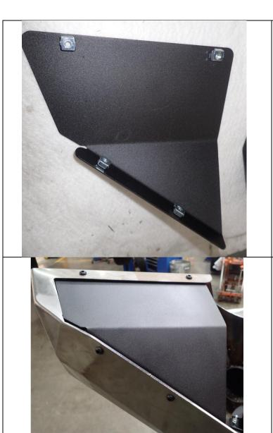
27. Fit 4x M6 Cage nuts to the inside of each wing panel.
