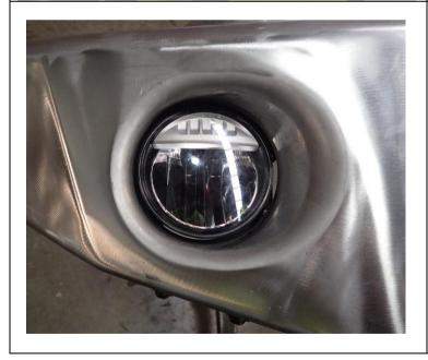
26. Adjust fog light so that it sits central to the fog light aperture in the bull bar.
