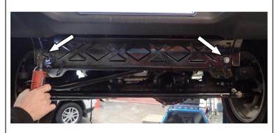
3. Remove 2x M10 SEMS from the steel front panel and discard.
