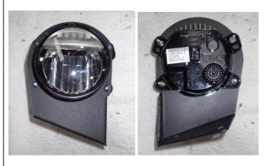
24. Loosely install front of fog lights to rear of mounting brackets using M4 fasteners supplied with fitting kit.
