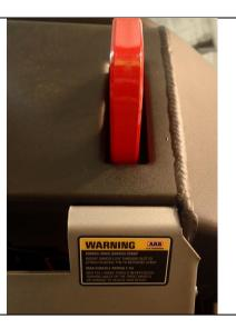
35. Fit recovery point decals to under panel directly below recovery points as shown.
