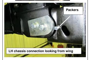
46. Insert 8 sets of M12 x 60 bolts, spring washers, flat washers and flange nut to holes drilled in side of chassis. On the outside face, the place washer is used over the large slot in the mounts. Do not tighten bolts.
