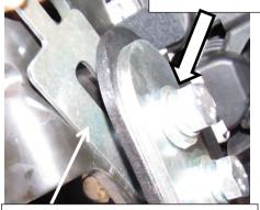
Fill any gaps between chassis and bar mount with packers before tightening bolts
