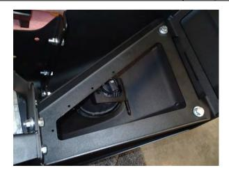
15. Fit wing braces using 4 x M10 SEMS bolts ,8x M10 washers and 4x M10 flange nuts and tighten the bolts
