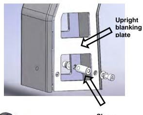
21. If outerframes are not fitted, fit blanking plates to uprights. M8 button head cap screws, stainless M8 spring washers and stainless M8 flat washers from either side.
