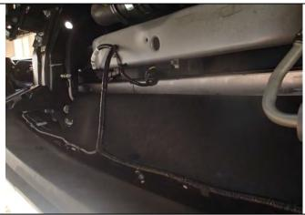
1. From behind the bumper un-plug and cut cables ties securing the fog light wiring loom
