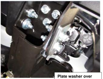
Plate washer over large slot on outside mount
