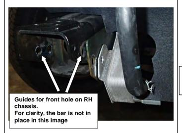
42. Once satisfied with the adjustment of the bar. Drill the pinning bolt locations in the sides of the mount brackets
