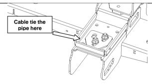
41. Cable tie the pipe detached at step 10 to mounting bracket hole shown in the image.
