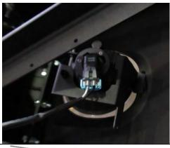
16. Connect fog light loom to the fog light and secure loom to wing brace using cable ties through holes on the wing brace.
