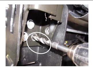
43. Drill the pinning bolt locations in the top face of the mount brackets.
