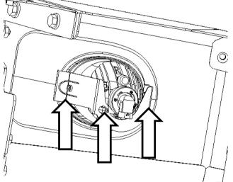
14. Slide fog lights into wings from the front and clip into position. RH side shown.
