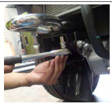
8. Remove tow hooks by unbolting 3 bolts from each side. Keep bolts as they will be used later.
