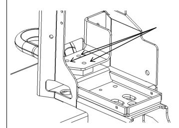
28. Fit tow hooks to bar using original fasteners and nut plates.
