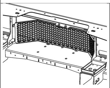
26. If no winch is fitted, attach mesh guard using six black M8 bolts, spring and flat washers and black M8 flange nuts.
