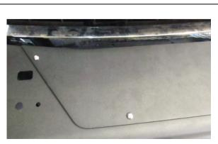
49. If not fitting a winch, fit panel to top face on bull bar using 4 x M6 dome head stainless steel screws, flange nuts and SS flat washers.
