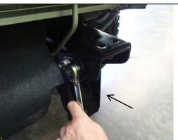
9. Remove brackets that are attached to chassis from either side. Remove and discard any fasteners and captive locking washers.
