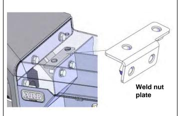
19. On Both sides, loosely fit weld nut plates to upright using 2 x M12 x 40 bolts, M12 spring washers and M12 flat washers, but do <u>not tighten</u>. Make sure that holes of top pan and weld nut plate are aligned.
