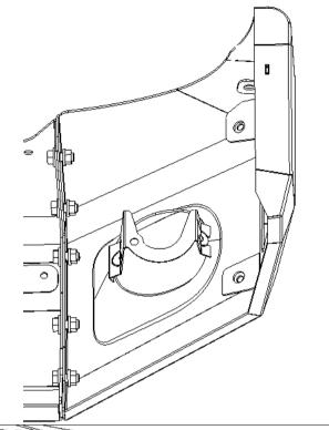
13. Fit each wing to bar using five sets of M12 x 35 fine thread bolts, M12 flat washers and M12 flange nuts. Align wings to centre section around the top and front face.
