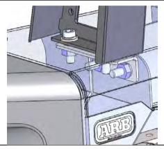
20. Loosely secure centre bar to top pan through weld nut plates from both sides using 4 x M12 x 40 socket head bolts, M12 spring washers and M12 flat washers. After alignment tighten all 8 bolts.
