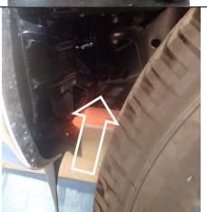
3. Unbolt the bumper brace at the chassis end.
