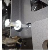
22. Position spacer in between bull bar mounting bracket and chassis
