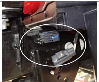
3. Disconnect fog light harness, located on the RHS chassis rail, access from wheel arch.
