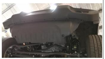
1. Remove plastic splash panel from underneath bumper by removing 2 lower screws and prying apart 8 plastic grommets,
