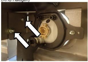
14. Secure fog light assembly to bull bar using M8 fasteners supplied with fog light fitting kit.
