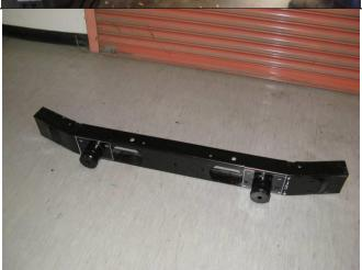
7. Remove steel impact beam from bumper.
