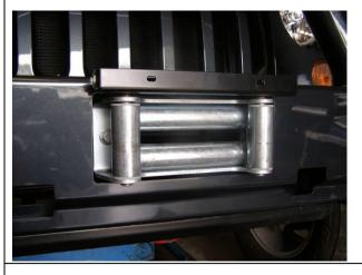
30. Fit the roller fair lead/hawse to the bull bar using M10 or 3/8" fasteners supplied with winch fitment kit.
