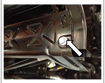
2. Remove front steel panel by removing both mounting bolts.
