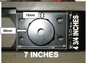
Note: If vehicle not equipped with steel impact structure (crush cans) as shown, ARB kit 3550240 is required for air bag compatibility. Skip to step 12.
