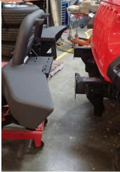
19. With the assistance of a friend or lifting device, present the deluxe bar to the vehicle.
