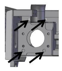
18. Position crush cans into mounting bracket openings located at the rear of the bar.
