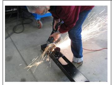
9. Carefully cut marked section using an angle grinder fitted with a cutting disc.
