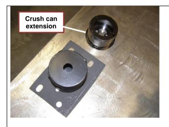
11. Attach crush can extensions supplied with bull bar to crush cans using 6x self-drilling screws supplied with fitting kit.
