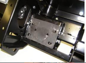
Note: To hold crush can / impact absorbers plate in position, smear a small amount of silicon onto mounting face.
