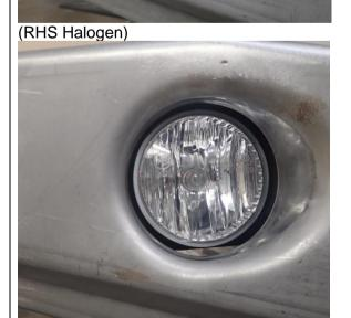
15. Adjust fog light so that it sits central to the fog light aperture in the bull bar.
