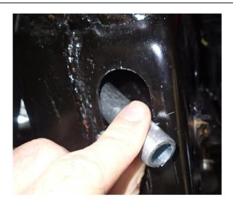
21. Assemble M12x82mm crush tube into lower section of chassis rail via the opening at the front.
