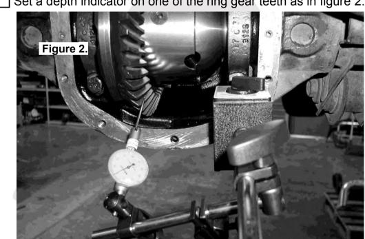
Set a depth indicator on one of the ring gear teeth as in figure 2.
