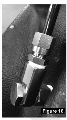
☐ Push the airline into the compression fitting body and screw the outer nut down onto it. Using a 12mm spanner, tighten the outer nut onto the compression fitting body.
