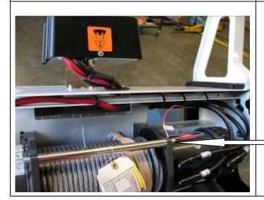
32. Fit all 3 cables to their correct terminals and tighten. Refer to Warn installation instruction when wiring up winch. Fit plastic boots over terminals. Cable tie cables to brace as per photo to clear of all moving parts. Fit ground wire under winch tie rod. ( See Photo )
