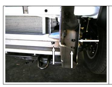
4. Fit bracket mounting assembly to front of vehicle using the 6 x 10mm studs to locate on.
