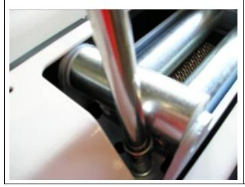
29. When all bolts are fitted and tighten, refit vertical roller pins back into roller fairlead and refit circlips.
