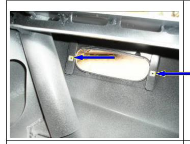
14 Fit white nylon plugs into square holes in light bracket.
