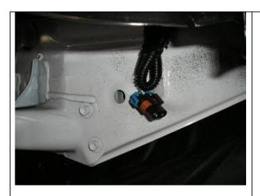
11. If vehicle is fitted with fog lights, remove globes from sockets and cable tie fog light loom to vehicle panel.
