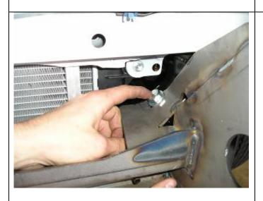
7. Fit M12 x 1.25P X 35mm (fine thread) bolt with 12mm flat washer through top rearward bracket passing through body mount.
