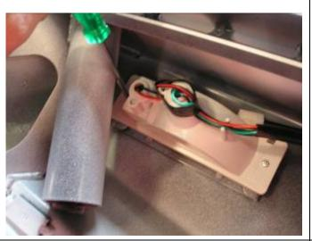
15. Align indicator/parker light above white nylon plugs and secure to bull bar using self tapping screws.
