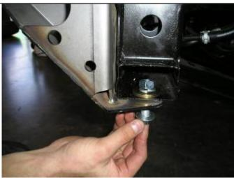
9. Secure lower fixing point by passing through lower bracket in a upward motion, using M12 bolt, 12mm flat washer and secure from the top using large gold coloured 12mm flat washer,12mm spring washer and M12 nut (fine thread) to each side of vehicle. When all bolts are fitted, tighten securely.
