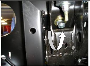
Secure from underneath using large 12mm gold coloured flat washer,12mm spring washer and M12 nut to both sides of vehicle.
