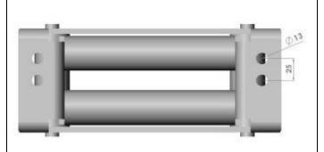
24. Drill two new 13mm holes in the roller fairlead provided in the kit, as shown on the adjacent picture.
