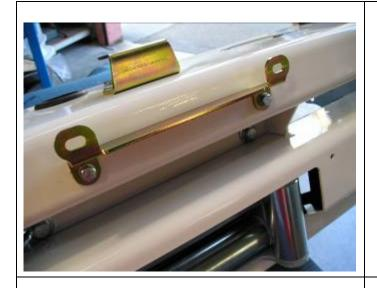
30. Fit number plate bracket to bar using M6 hardware.
