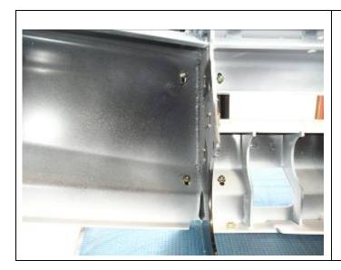
18. Fit buffers to bar and secure from inside of bull bar using M6 flange nuts. Six to each side of vehicle.
