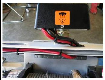
31. Fit control box to control box bracket and pass cables through rubber grommet.
