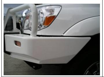
35. Align bull bar so there is a 15mm to 20mm gap around periphery under front vehicle panels, then tighten all bolts securely.
