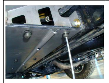
2. Fit the skid plates to the rocker rails using the M8 x 20mm button head socket screws, M8 flat black washers and M8 black spring washers.
