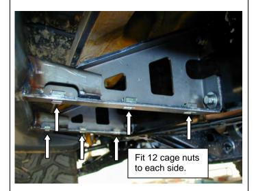
1. Fit the 24 cage nuts into the square holes in the chassis brackets of the rocker rails.
