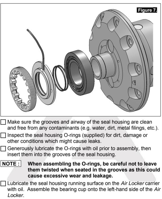
Carefully install the seal housing by sliding it all of the way onto the bearing journal with a gentle twisting motion. (Note the orientation of the seal housing.) This will allow the O-rings to engage gently (Fig. 7.).
