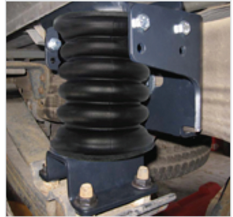
Typical SSR-101 installation with standard lower bracket *SumoSprings Black -47 used in photo
