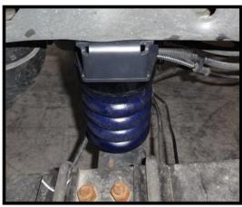
Refer to SumoSprings application guide for part selection www.supersprings.com [Tech Iline 866-898-0720] 10/21/15 SumoSprings enhance load carrying capability, handling & towing. Never exceed vehicle manufacturer's GVWR rating.
