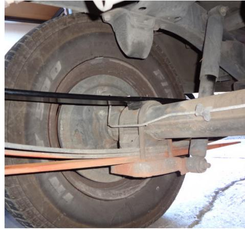
SuperSprings are installed on top of axle.
