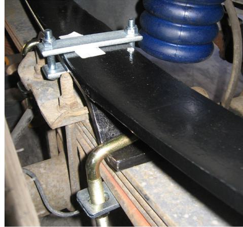
SuperSprings are installed on top of MTKT mounting kit.
