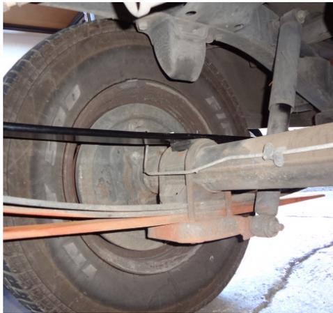
SuperSprings are installed on top of axle.
