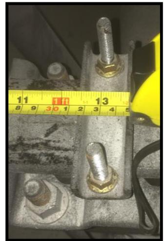
**Step 4:** Position the shackle on the front of the SuperSpring so that it is directly behind the sway bar link. (see picture at right). **Ensure head of upper shackle bolt is clear of sway bar link!**
