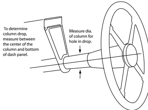
Column drops have a hinged mount to accommodate various mounting angles. Column drops are split at column hole for mounting, bolts are up through bottom. Includes two bolts and lock washers for attaching to dash.
