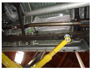
Step 3. Only the Crew Cab Long Bed configuration will require the supplied 12.5 Extension Pipe, Install this to Inlet Pipe Assembly if required using the supplied 3.50" clamp then attach the Muffler Assembly to the Extension Pipe. If the 12.5" Extension Pipe isn't used attach the Muffler Assembly directly to the Inlet Assembly with a supplied 3.50" clamp.
