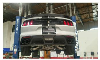
**Step 8.** Once a final position has been chosen for the new exhaust system, evenly tighten all clamps from front to rear using the torque specifications on page one of the instructions. Inspect all fasteners after 25-50 miles of operation and re-tighten if necessary.
