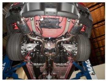
**Step 7.** Loosely install the Muffler Assemblies using the supplied clamp. Attach the welded hangers to the rubber insulators. Re-attach both electrical connectors to the exhaust valve motors.
