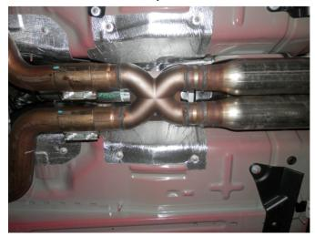
**Step 2.** Next loosen the clamps at the vehicles catalytic converter outlet pipes. Working from front to rear disengage all welded hangers from the rubber insulators. Retain all mounting hardware as it will be needed to mount your new MAGNAFLOW system.
