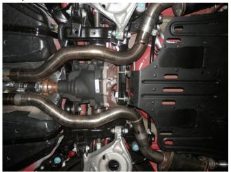
**Step 6.** Attach both Over Axle Pipes to the X-Pipe Assembly using the supplied clamps. Engage the welded hangers to the rubber insulators.
