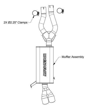
Step 1:(Carefully read all instructions before installation) Begin removing the OEM exhaust system by first unbolting both clamps attaching the muffler assembly to the catalytic converter outlet pipes. Remove the mounting hardware securing the muffler. Working front to rear remove the system. Be sure to retain and not to damage all mounting hardware as it will be needed to mount your new MAGNAFLOW exhaust system.
