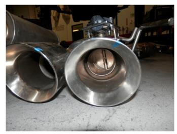
**Step 4.** Before installing your new exhasut system attach the OEM valve motors to each valve using the supplied M5 hardware. The alignment spring on the motor will need to be engaged into the keyway slot of the new valves.
