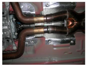
**Step 5.** Install the X-Pipe Assembly to the OEM slip clamp. Engage the welded hangers to the rubber insulators. Leave all clamps loose for final adjustment of the system.
