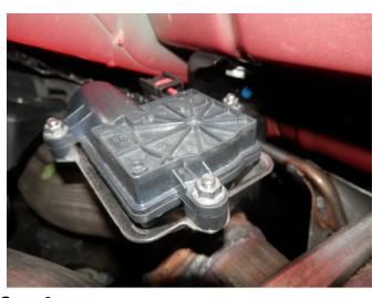
**Step 3.** Once the OEM system has been removed undo three nuts attaching each exhaust valve motor to the valve and remove.
