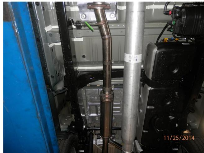
**Step 4.** If your vehicle has a Crew Cab/Standard Bed configuration you will need to include the supplied 14.50" Extension Pipe between the Inlet Pipe Assembly and the Muffler. For Crew Cab/Short Bed and Extended Cab/Standard Bed the Extension Pipe is omitted. Next loosely attach the Muffler to the Inlet Pipe Assembly using the supplied 3.00 clamps.
