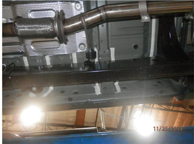
**Step 3.** Begin installing of the new system by attaching the Inlet Pipe Assembly to the flange re-using the OEM fasteners and inserting the hanger into the rubber insulator.
