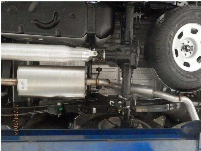
**Step 1.** To remove the OEM system you will need to unfasten the two bolt flange located behind the flex pipe. Working rearward (with the exhaust supported) extract the hangers from the rubber insulators and remove the OEM exhaust. Do not discard or damage the rubber insulators or fasteners as they will be used to install the new exhaust system.
