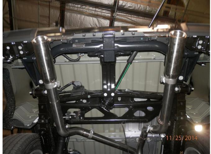
**Step 7.** Install the two Clamp-On Tips using the supplied 2.50" clamps.
