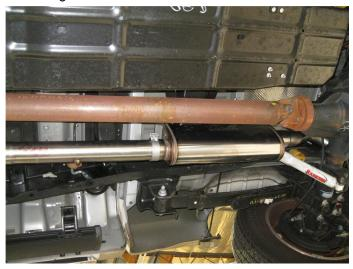
**Step 4.** Install both the Muffler Assembly and Tail Pipe Assembly using the supplied 3.50" clamps. Locate the welded hangers to the OEM rubber insulators.
