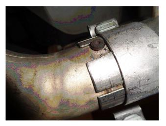
Step 2: To install the MagnaFlow Muffler Assembly slide the inlet onto the OE outlet making sure to align the slot with the peg on the outlet pipe. Secure with the supplied 3.50" clamp.
