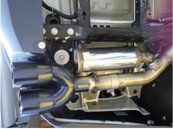
**Step 6.** Complete the installation by attaching both Tailpipe Assemblies to the Y-Pipe Assembly using the Supplied 2.50" clamps and engaging the welded hangers to the rubber insulators.
