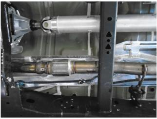
**Step 2.** There are two inlet pipe assemblies supplied in this kit to accommodate the 5.3 and 6.2L engines. Select the appropriate inlet for your engine configuration. The assembly with the larger inlet flare will be for the 6.2L engine. Begin the install by fastening the Inlet Pipe Assembly to the outlet of the OE system using the OE clamp (Leave all clamps and fasteners loose for final adjustment of the complete system.)
