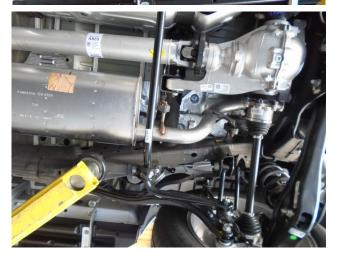
**Step 1.** To remove the OE exhaust system you will to need to remove the spare tire, heat shield and sway bar. Unfasten the clamp attaching the OE inlet pipe assembly to the catalytic converter. Do not damage or discard the inlet pipe clamp or rubber insulators as they will be re-used to mount the new system. Working front to rear disengage the hangers from their rubber insulators and remove the exhaust from the vehicle.
