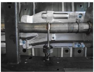
**Step 3.** Attach the Extension Pipe Assembly to the Inlet Pipe Assembly with a supplied 3.00" clamp. Engage the welded hanger to the rubber insulator.
