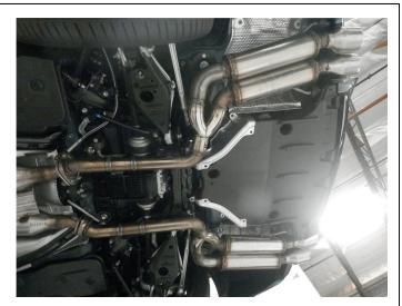
**Step 2.** Begin installation of the new system by fastening the inlet flanges of each Muffler Assembly to the outlet flanges of the catalytic converters using the OEM spring and bolt along with the supplied hardware. Locate the each welded hanger into the OEM rubber insulator.
