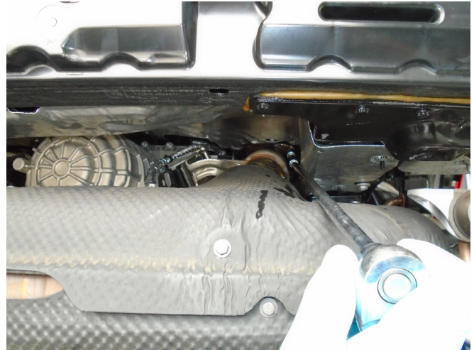
Step 15. The exhaust inlets connected to the catalytic converters are now accessible. Remove (2) 15mm hex nuts from the drivers side and (3) 13mm hex nuts from the passengers side inlet flanges.
