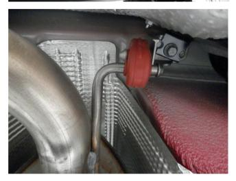
**Step 1.** Begin removal of the OEM system by loosening at the inlet of the Resonator and removing the black tubular cross brace. You can then disengage the welded hangers from the rubber insulators, working rearward finish removing the system. Do not damage or discard the rubber insulators or OEM clamp as they will be re-used to mount the new system.
