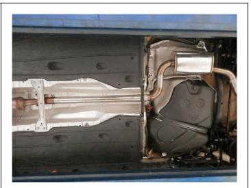
**Step 2.** Begin installation of the new system by attaching the Inlet Pipe to the factory outlet using the OEM clamp. and fit the hangers into the rubber insulators. Leave all clamps loose until final adjustment. Next Install the Muffler Assembly using the supplied 2.50" clamp and fit the welded hanger on the assembly to the previously un-used hanger on the underside of the vehicle using the supplied rubber insulator.
