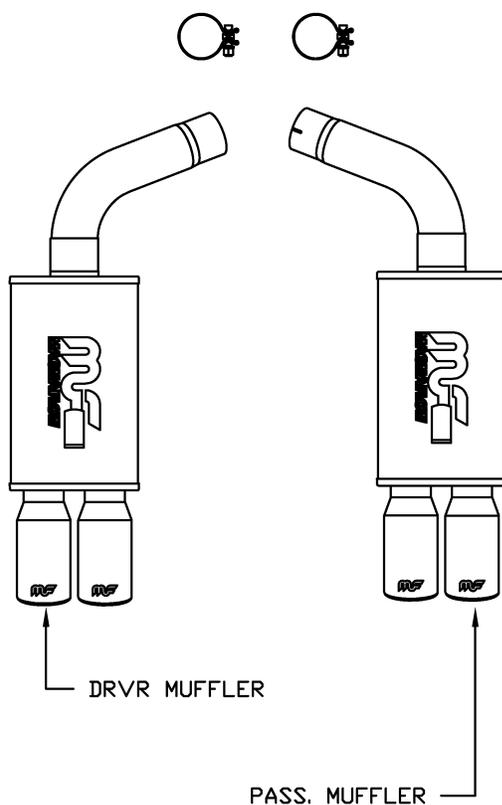
**Step 2:** For packaging, the bolt-on mounting brackets are installed backwards on the mufflers. Unbolt them from the mufflers and insert them into the OEM rubber insulators under the rear bumper. Fit the inlet pipes of the mufflers over the ends of the OEM exhaust pipes and fasten them with the supplied 2.75" clamps. Leave all fasteners loose for final adjustment of the system. Hold the mufflers in position and bolt them to mounting brackets you mounted into the OEM rubber insulators.
