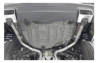
**Step 3.** Attach the Mid-pipes to the Resonator Assembly with supplied 2.50 Clamps and fit hangers into rubber insulators. Remember to re-attach the ground strap to the hanger. At this point you have two options for tips. Magnaflow supplies a straight tip setup that can be run into the existing valance surround and held in place with hangers and the installation is complete.
