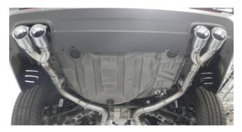
**Step 4.** We also supply a Quad tip setup that requires removing the tip surrounds located in the valance. Once removed the quad tips are routed into the openings.
