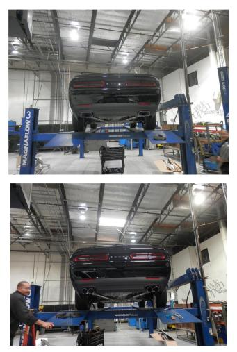
Step 5. Once a final position has been chosen for the new exhaust system, evenly tighten all clamps from front to rear using the torque specifications on page one of the instructions. Inspect all fasteners after 25-50 miles of operation and re-tighten if necessary.
