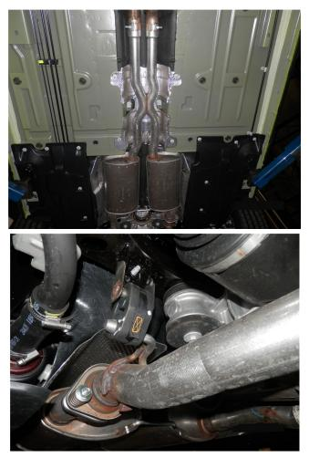
**Step 1.** To begin the removal of the OEM system you will need to unfasten the X-Pipe inlets at factory clamp locations. Next un-clip the ground strap from the passenger side muffler hanger. Working rearward (with the exhaust supported) extract the hangers from the rubber insulators and remove the OEM exhaust. Do not discard or damage the rubber insulators as they will be used to install the new exhaust system.
