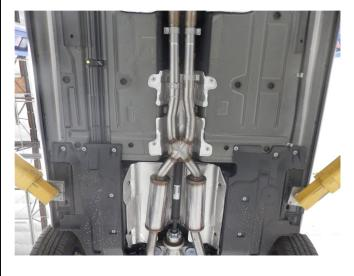
**Step 2.** Begin installing of the new system by attaching the Driver and Passenger side (Passenger is the longer of the two pipes) inlet pipes to the outlets of the OEM system using the supplied 2.25" clamps. Next attach the Resonator Assembly to the inlet pipes with supplied clamps and insert the hangers into the rubber insulators.
