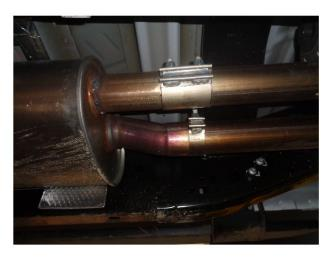
**Step 2.** Next loosen both band clamps attaching the rear muffler subassembly to the inlet muffler assembly. Disengage all welded hangers from the rubber insulators. The muffler subassembly may now be removed.
