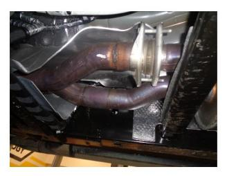
**Step 3.** Finally remove the OEM inlet muffler assembly by unbolting the inlet at the driver side flange junction and loosening the band clamp on the passenger side inlet pipe. Remove the inlet muffler asembly. You are now ready to install your new
