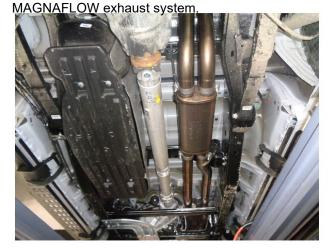
**Step 4.** Install the Muffler Assembly by attaching the inlet nipples to the outlets of both Inlet Pipe Assemblies. Loosely secure using the supplied clamps. Engage the welded hanger to the rubber insulator.
