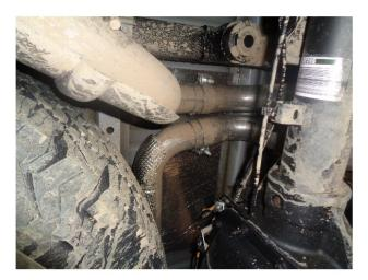
**Step 1.** Begin removal of the OEM exhaust system by loosening the band clamps attaching the tail pipe assemblies to the over axle pipes. Disengage all welded hangers from the rubber insulators and remove both tail pipes. Retain all mounting hardware as it will be used to install your new system.
