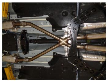
**Step 3.** Install the new X-Pipe Assembly by loosely bolting it to the catalytic converter outlets using the OEM gaskets and fasteners.
