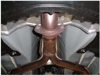
**Step 2.** Unbot the flanges coupling the inlet pipe assembly to the resonator assembly. You may also unbolt the muffler assembly to ease the system removal process. Working front to rear disengage all welded hangers from the rubber insulators. Retain all mounting hardware as it will be needed to install your new MAGNAFLOW system.
