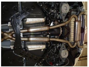
**Step 4.** Next loosely attach both Resonator Assembles to the X-Pipe Assembly outlets using the supplied clamps. Locate both welded hangers to the rubber insulators.
