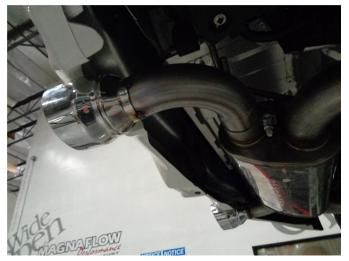
Step 6. Install both Tail Pipe Assemblies to the Muffler Assembly. Loosely secure using the supplied clamps.
