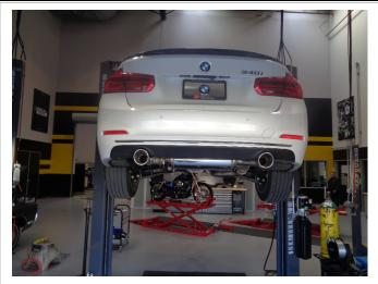
Step 6: Once a final position has been chosen for the new exhaust system, evenly tilgten all clamps from front to rear using the torque specifications on page one of these instructions. Inspect all fasteners after 25-50 miles for operation and re-tighten if necessary.
