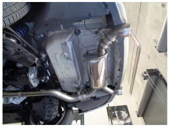
Step 5: Install the Muffler Assembly by attaching the inlet to the Extention Pipe. Loosely secure using the supplied clamp. Locate both welded hangers to the OE rubber insulators. Reattach the electical connector plug to the valve motor and reinstall the cross member.
