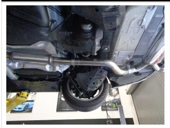
Step 4: Loosely attach the Resonator Assembly Inlet to the Inlet Pipe Assembly outlet with the supplied clamp. Install the Extention Pipe to the Resonator Assembly the same way.
