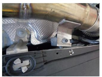
Step 3: Begin the installation process by loosely attaching the Inlet Pipe Assembly to the catalytic converter outlet using the clamp you removed from the OE system. Locate the hanger bracket to the OE hanger location and loosely secure using the OE hardware.
