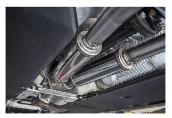
Step 2: Begin installation of the new system by fastening the Resonator Assembly inlet to the flange outlet using the OE fasteners (Leave all clamps and fasteners loose for final adjustment of the complete system.)
