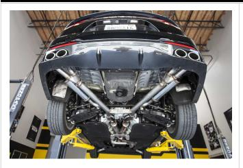
Step 4: Once a final position has been chosen for the new exhaust system, evenly tighten all clamps from front to rear using the torque specifications on page one of these instructions. Tighten fasteners for Muffler brace and install factory underbody brace. Inspect all fasteners after 25-50 miles for operation and re-tighten if necessary.
