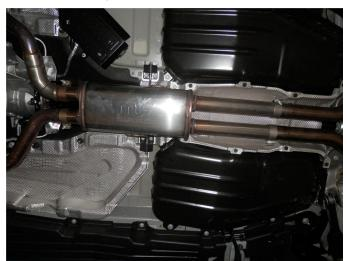
**Step 2.** Begin installation of your new MAGNAFLOW system by attaching the Inlet Muffler Assembly to the two catalytic converter outlet pipes. Loosely secure using the supplied 2.36" clamps. Fit the hangers into the rubber insualtors. Leave all clamps loose until final adjustment.
