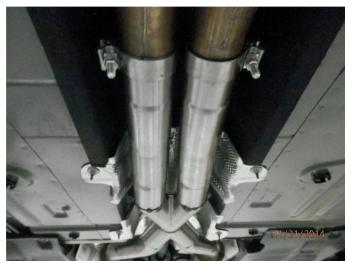
**Step 6.** Begin installation of the new system by slipping the inlet tubes corresponding with your vehicle. Loosely securing associated clamps provided. Next slip on the X-Pipe Muffler Assembly over the inlet tube adaptors. Loosely secure using two of the suppled 3.00" clamps. Orientation of the Muffler Assembly can be confirmed by the MF logo being "upright" after installation.
