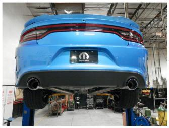
**Step 9.** Once a final position has been chosen for the new exhaust system, evenly tighten all clamps from front to rear using the torque specifications on page one of the instructions. Inspect all fasteners after 25-50 miles of operation and re-tighten if necessary.
